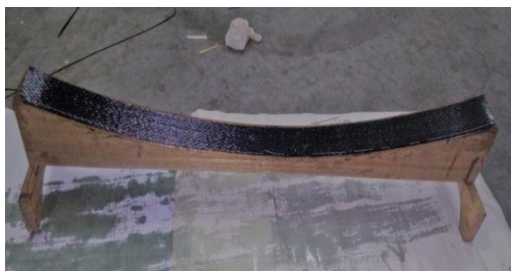
Fig.3 Laying of the cloth on mould
