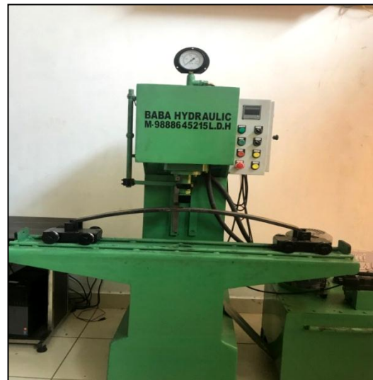
Fig.9 Fatigue testing of composite leaf spring
