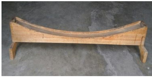
Fig.1 Mould for Composite Leaf Spring
