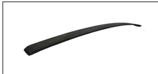
Fig.6 Finished carbon epoxy composite leaf spring
