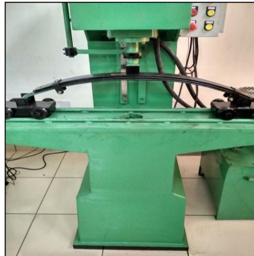
Fig.8 Fatigue testing of steel spring
