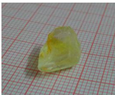
Fig. 1 Harvested Crystal of Picric Acid Doped KDP
