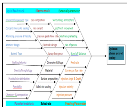
Fig. 5 Influence of the parameter to optimum plasma sprayed coating
