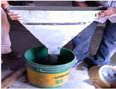
Fig. 3 Experimental setup of V Funnel Test
