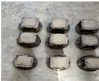
Fig. 4Casting of Cubes
