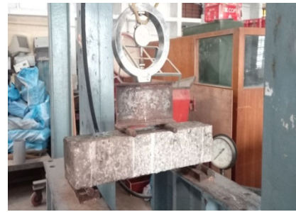
Fig. 10 Flexural Strength of Prism using Two Point Loading
