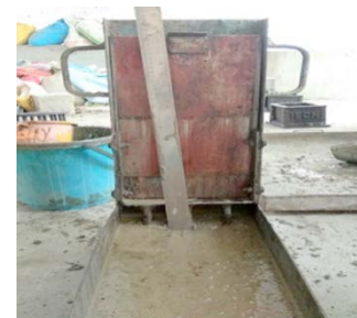
Fig.2 Apparatus for L BOX Test
