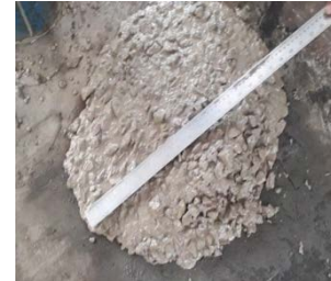
Fig. 1 Flow Test on Geopolymer Concrete
