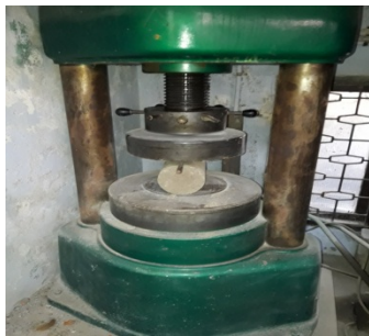
Fig. 8 Split Tensile Test of Cylinder
