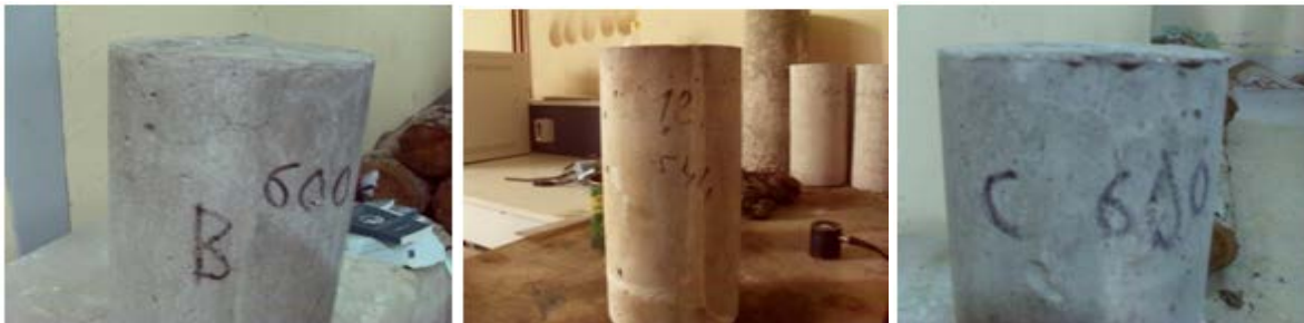
Fig.3 Appearance of significant cracks after 600 °C
