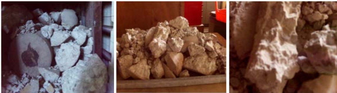
Fig. 6 Explosive Burst Of HPC2 To 544 °C
