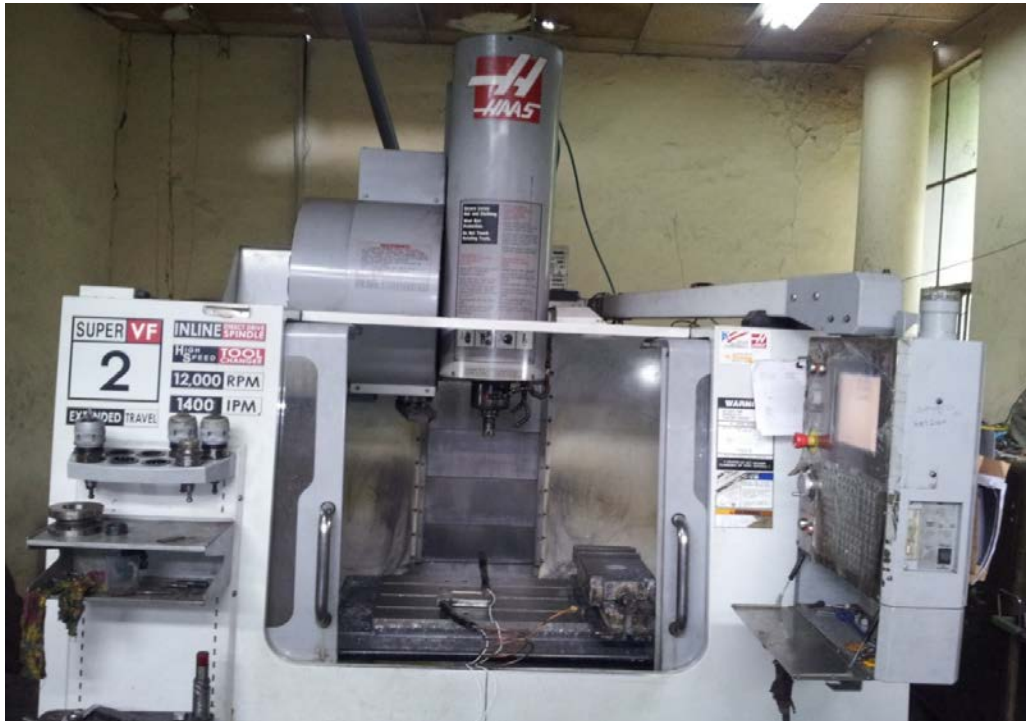
Fig. 1.3: Vertical milling machine used for FSP[11].
