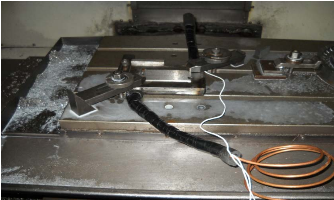
Fig. 1.2: Fixture clamped on the bed of CNC vertical milling machine[11].
