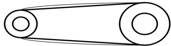
Fig. 3 Buckling on the connecting rod.
