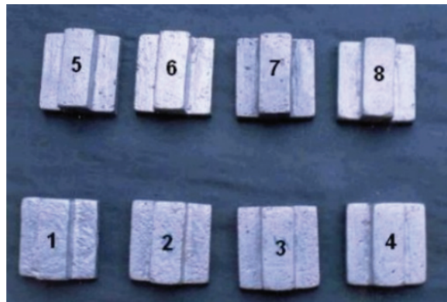
Fig 3 Photograph of Aluminum alloys sand castings
