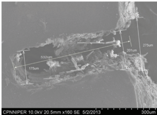
Fig.11 SEM of a slicing work-piece of e-glass fibre epoxy composite using 200 µm brass wire
