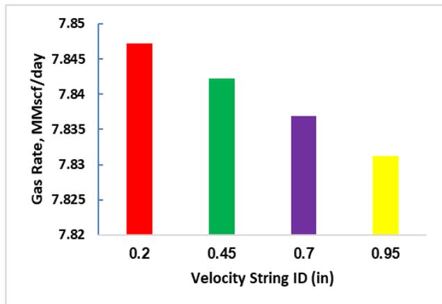
Fig. 7 Gas production rate for different strings diameter at 0.1 mass percent surfactant concentration
