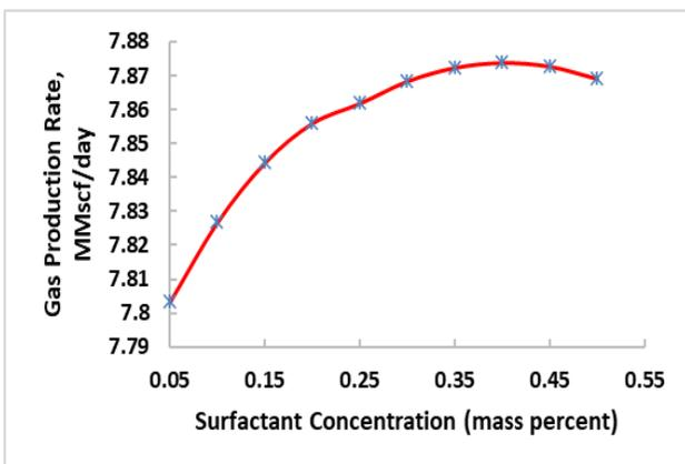
Fig. 4 Gas production rate against surfactant concentration
