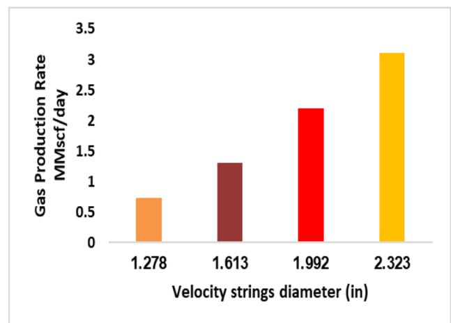
Fig. 6 Gas production rate against velocity string's diameter
