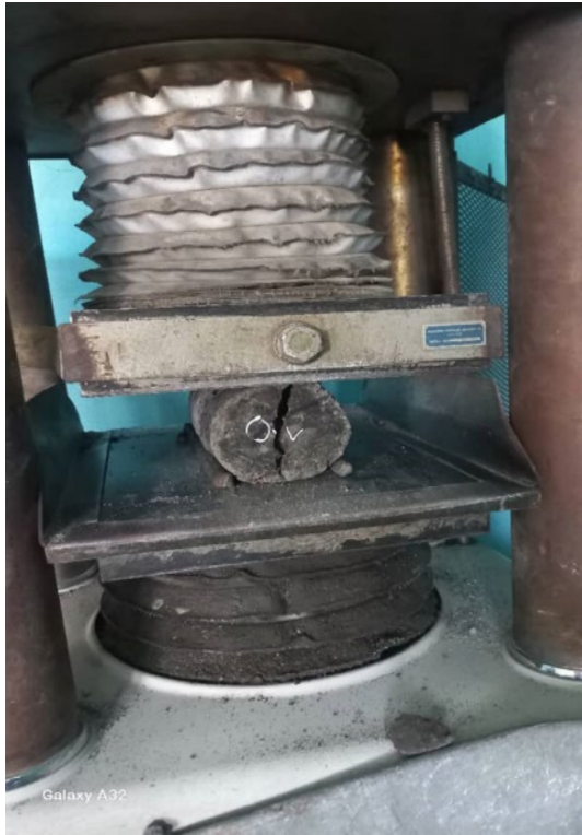
Fig. 1 A test of split tensile resistance is being done
