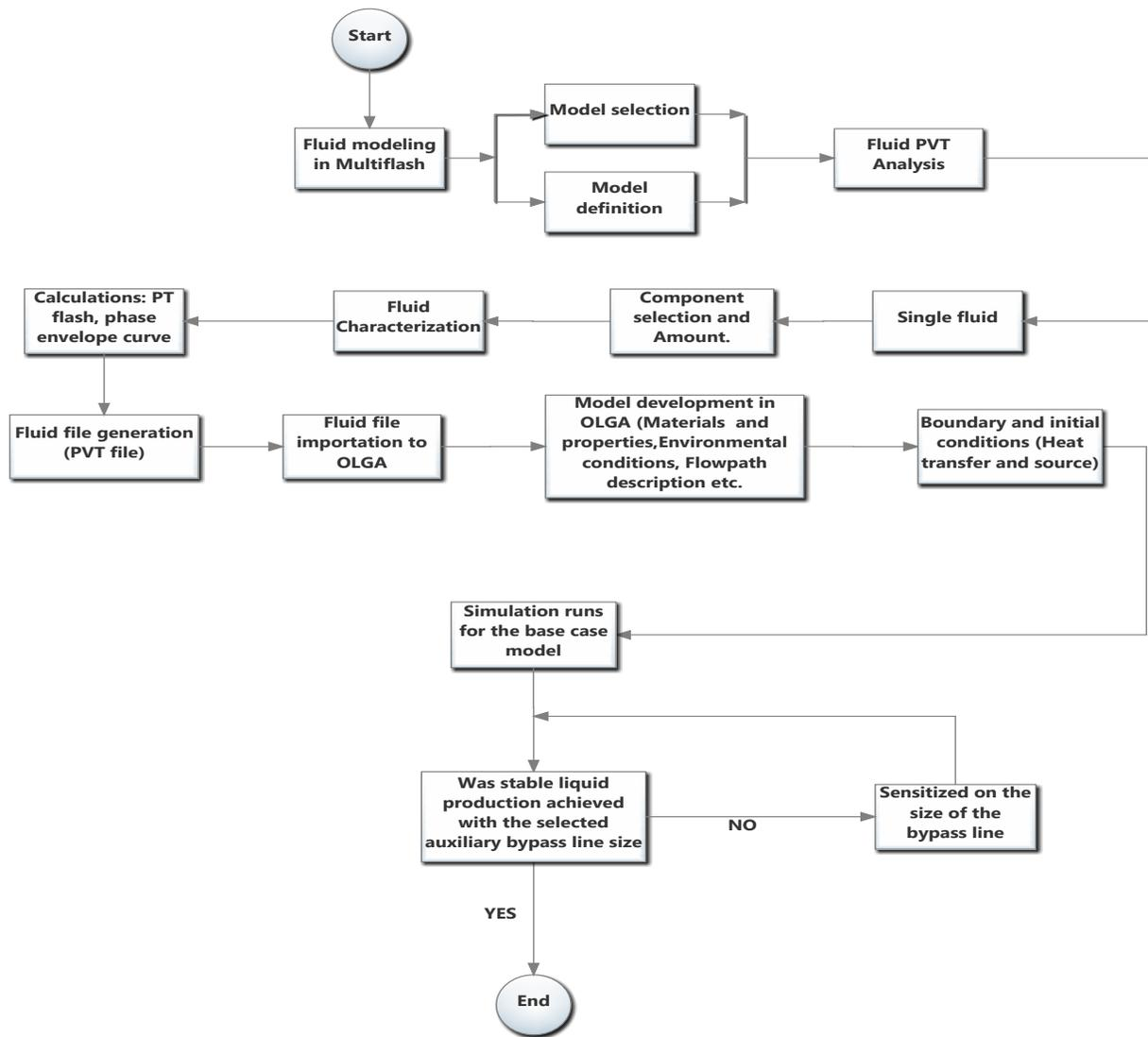
Fig. 1 Simulation workflow
