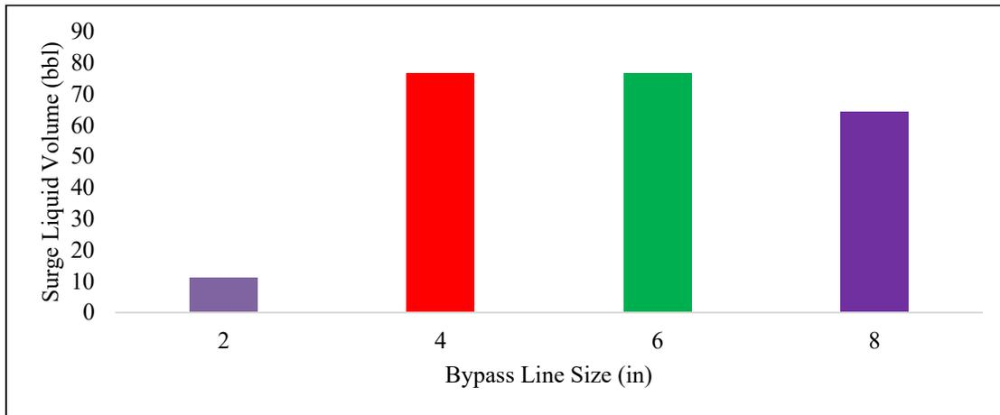
Fig. 8 Surge volume for different bypass line
